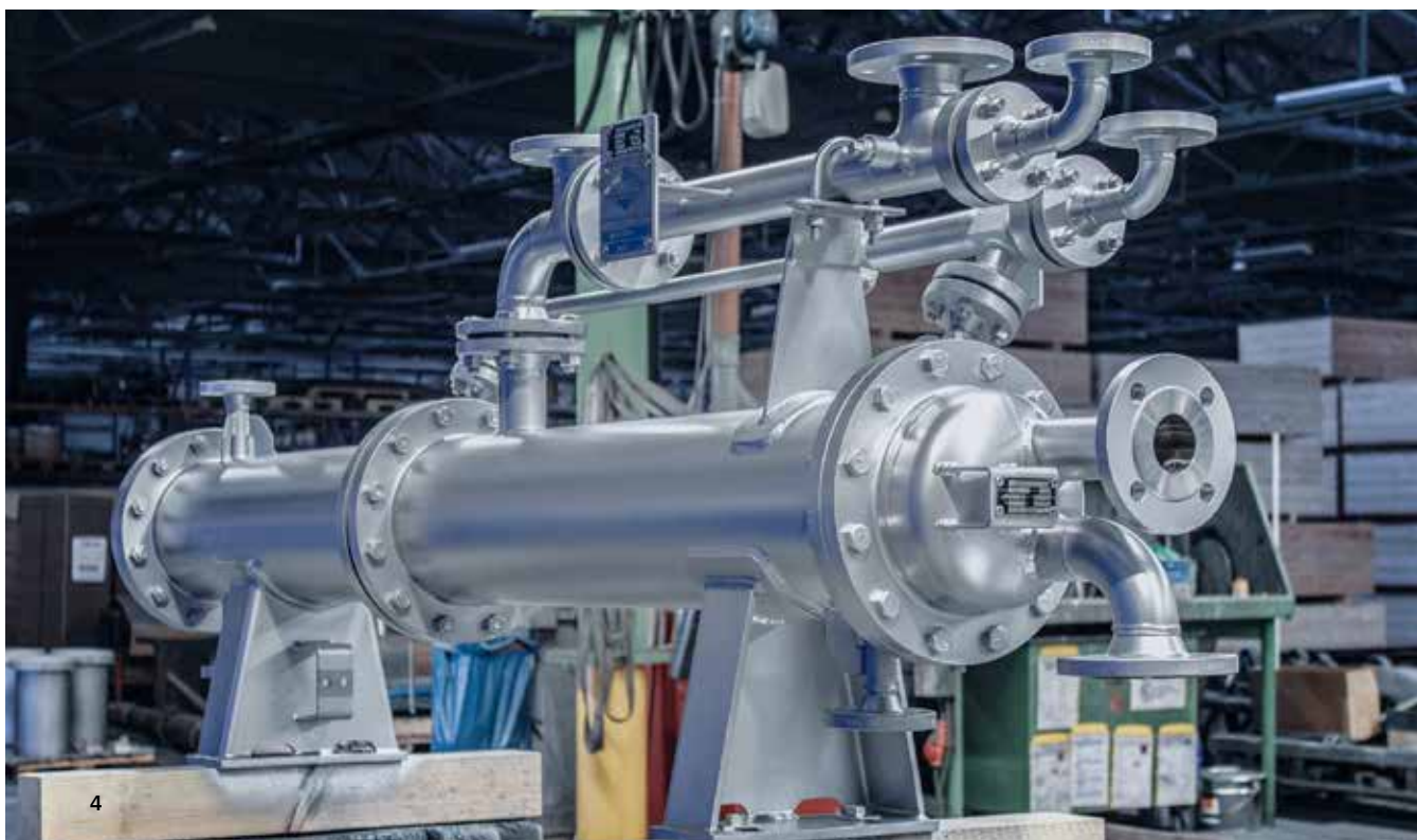
Two-stage, steam jet vacuum system with a surface condenser after final assembly
